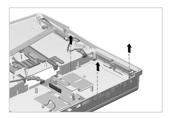
Figure 7-22. Removing the MultiBay Assembly Screws
